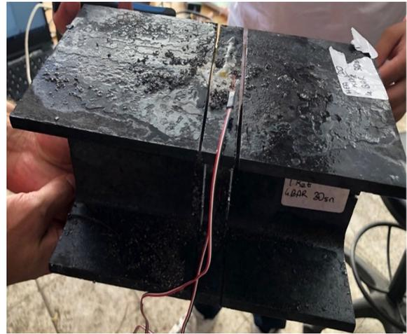
Fig. 3. Section with cutting method applied
