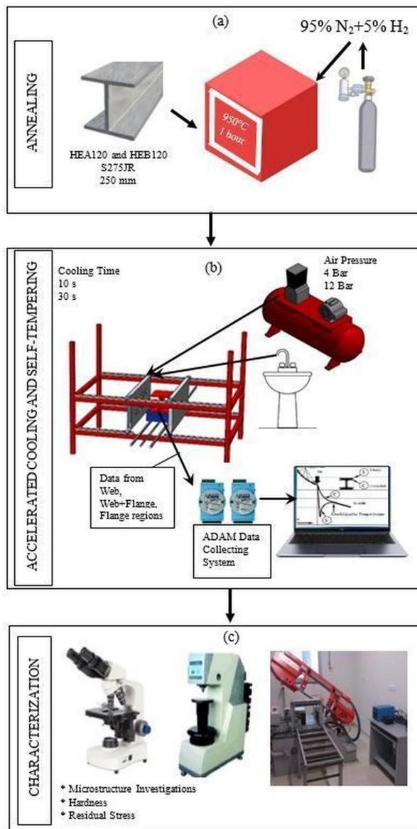
Fig. 1. Experimental flow diagram for a) annealing heat treatment, b) AC-ST process and c) characterization of the HEA120 and HEB120 sections
