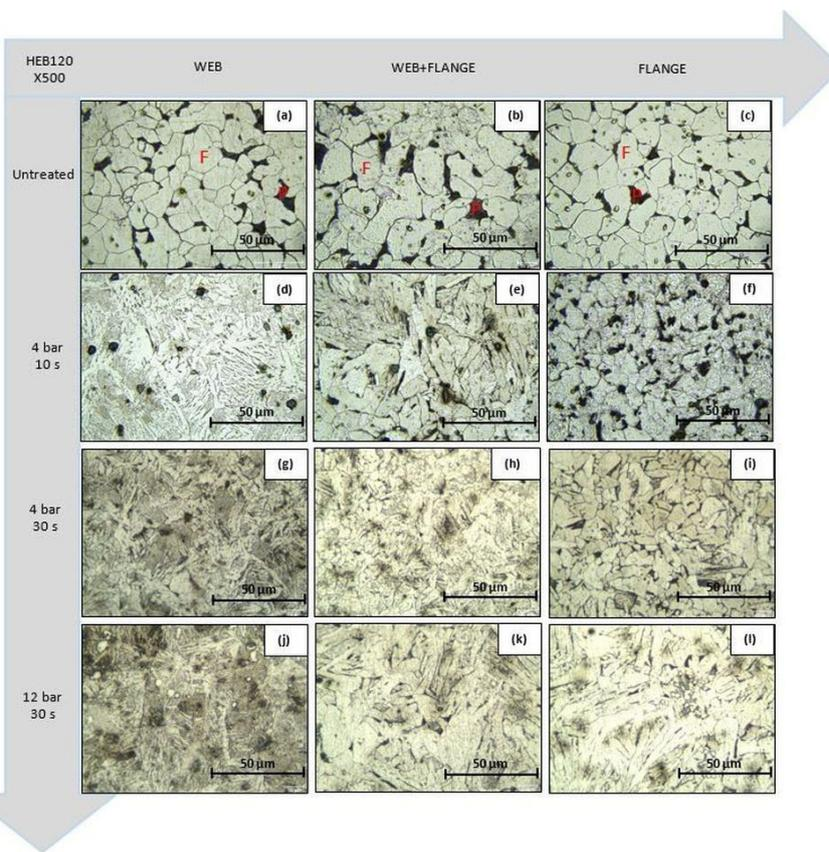
Fig. 8.  $\times 500$  magnification cross-sectional images in the web, web+flange and flange regions of the AC-ST HEB120 sections for different parameters (pressure and cooling time). Abbreviations: F: Ferrite, P: Pearlite
