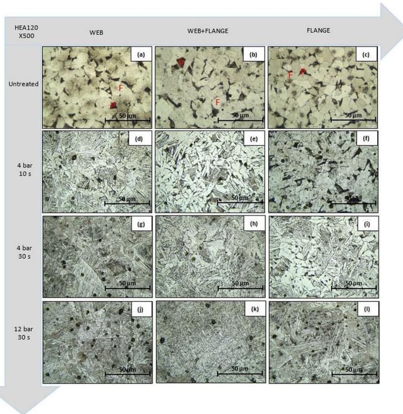
Fig. 7.  $\times 500$  magnification cross-sectional images in the web, web+flange and flange regions of the AC-ST HEA120 sections for different parameters (pressure and cooling time). Abbreviations: F: Ferrite, P: Pearlite
