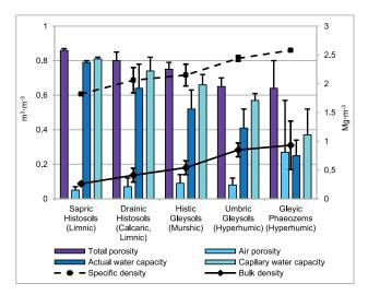
Fig. 3. Physical properties of organogenic layers of studied post-bog soils on Holocene carbonate limnic deposits in NW Poland; source: own study
