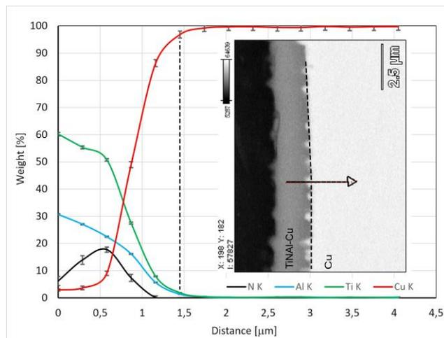
Fig. 7. Linear chemical composition for AlTiN/Cu boundary after 60 min / 750 °C, correspond to Figures 5b and 6b
