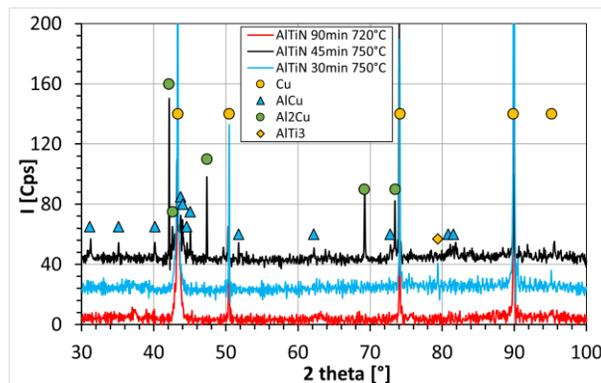
Fig. 9. The XRD diffraction on surfaces of the tested samples after exposure to different conditions, using copper lamp with a wavelength  $\lambda = 1.54$  [Å]
