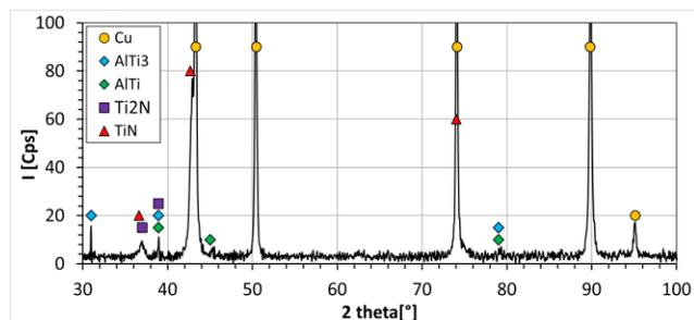
Fig. 4. The XRD diffraction for nitride protective coatings AlTiN (55/45 at.%) on the copper substrate, using copper lamp with a wavelength  $\lambda = 1.54 \text{ [\AA]}$
