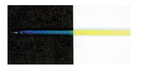
A glass fiber made of sodium borophosphate glass, doped with silver nanoparticles, exhibiting different colors depending on the light: against a bright background it is seen in transmitted light, whereas against a dark background it is seen in reflected light
