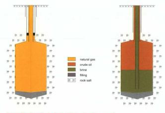
Generalized method of operation of underground storage caverns in salt diapirs
