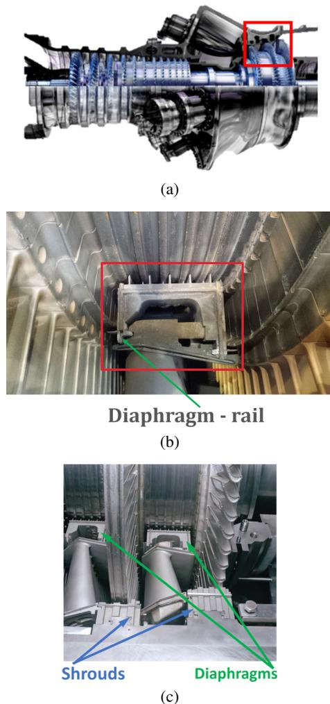
**Fig. 1.** Cross overview of the gas turbine (a); Cross-section through turbine shell (b); Power nozzle assembly with marked diaphragm (c)
