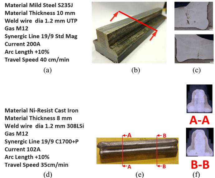
**Fig. 4.** Development of process parameters for diaphragm additive repair, welding parameters used in the development phase (a), additive mockup using (a) parameters (b), cut ups of (b) printout (c), welding parameters used in the development phase (d), additive mockup using (d) parameters (e), cut ups of (e) printout (f)
