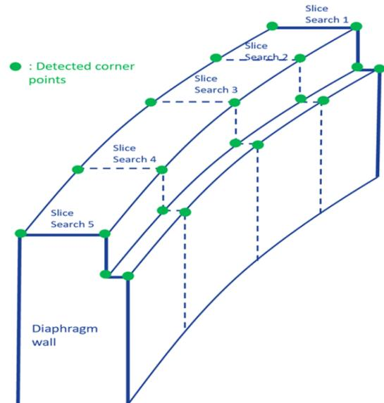
Fig. 6. Process of creating radial arc tool path along the diaphragm rail
