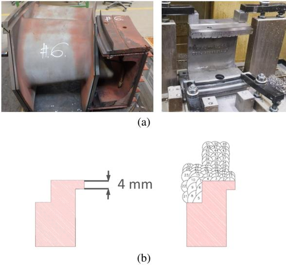
**Fig. 7.** Diaphragm assembly as received by Service Center (a) part after initial machining (a), cross section of the diaphragm after initial machining and different stages of cladding a worn diaphragm rail (b)
