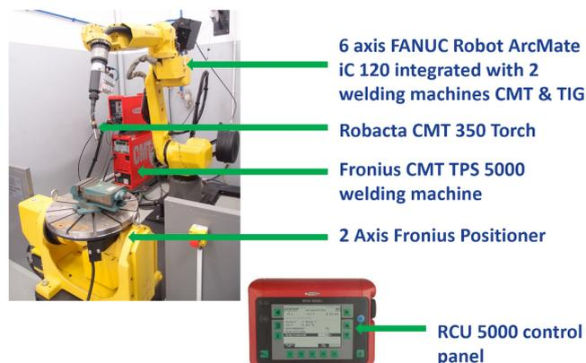
**Fig. 3.** Workstation with an Industrial robot FANUC ArcMate120iC, 2 axial positioner (Fanuc) and TPS 5000 CMT welding source (Fronius)
