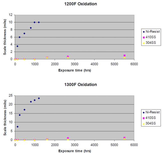
**Fig. 2.** Oxidation curves for 304SS, 410SS, Ni-Resist
