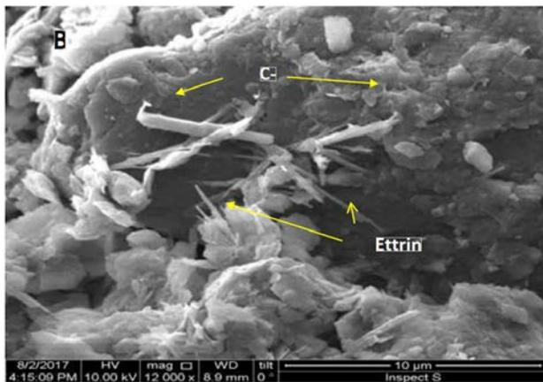
Fig. 6. SEM images for treated soil
