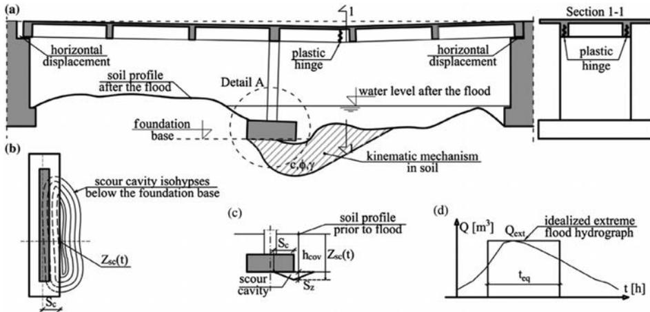
Fig. 1. (a) Bridge failure mode in the longitudinal direction; (b) a local scour cavity at the affected pier foundation; (c) detail a – the cavity approximation; (d) an idealized extreme flood hydrograph [8]
