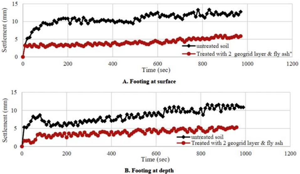
Fig. 10. Settlement against time for treated and untreated with fly ash and two geogrid layers models with velocity = 6 mm/sec and various depth
