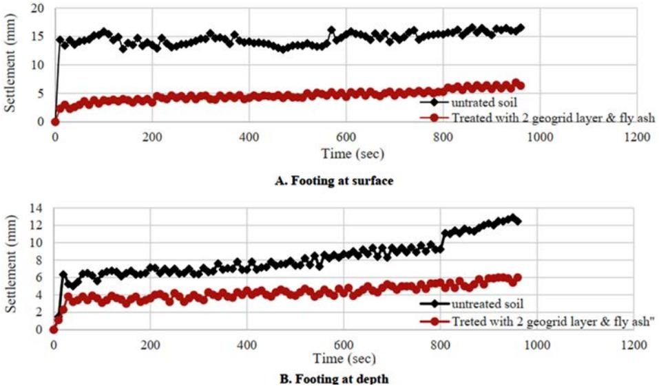
Fig. 9. Settlement against time for treated and untreated with fly ash and two geogrid layers models with velocity = 9 mm/sec and various depth
