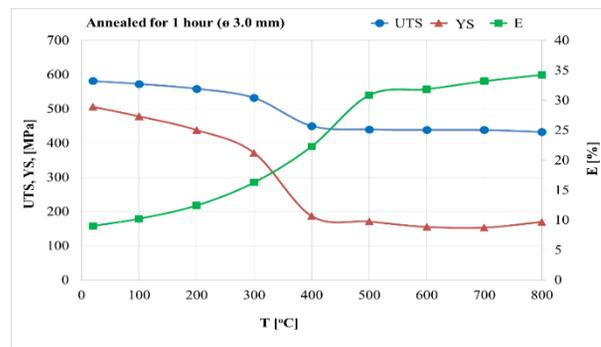
Fig. 4. Annealing curves for wires with a diameter of 3.0 mm annealed for 1 hour at different temperatures
