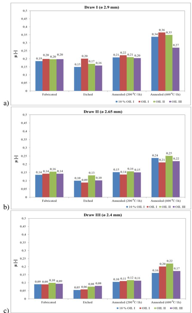
Fig. 7. The calculated coefficient of friction based on Tarnawski formula for drawn wires with a diameter of 2.9 (a), 2.65 (b) and 2.4 (c) using different lubricants
