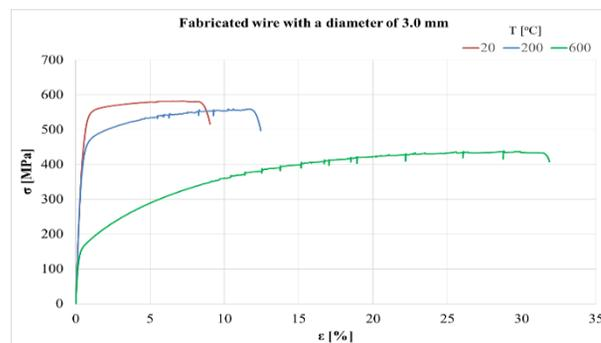
Fig. 5. Stress-strain curves for wires with a diameter of 3.0 mm not annealed ( $20^\circ\text{C}$ ), annealed at 200 and  $600^\circ\text{C}$  for 1 hour
