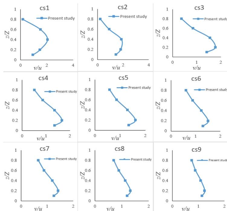
**Fig. 7.** Velocity profile for alternative design 4 – test No. 1; cs1–cs9 = chosen sections from 1 to 9, as in Fig. 2,  $z/Z$ ,  $v/u$  as in Fig. 3; source: own study
