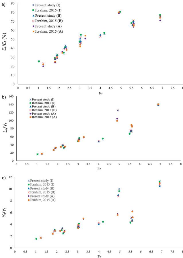
**Fig. 5.** Relationship between Froude's number ( $Fr$ ) and: a) relative energy losses, b) relative length of jump, c) submergence ratio;  $E_L$ ,  $E_1$ ,  $Y_1$ ,  $Y_3$ ,  $L_{sj}$  as in Fig. 4; source: own elaboration based on present study and Ibrahim (2015)
