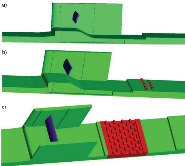
Fig. 1. Geometric shape of: a) group A, b) group B, c) group I; source: own elaboration made in Flow-3D by Flow Science (2014)
