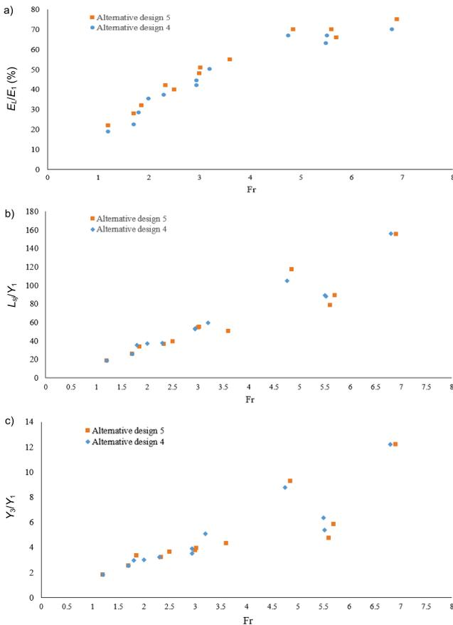
**Fig. 8.** Relationship between Froude's number (Fr) and: a) relative energy losses, b) relative length of jump, c) submergence ratio;  $E_L, E_1, Y_1, Y_3, L_{sj}$  as in Fig. 4; source: own study
