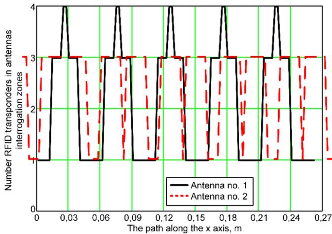
Figure 15: Number of transponders in the robot antennas interrogation zone for the square grid
