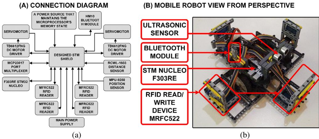
Figure 3: (a) Simplified connection diagram of robot components, (b) view of the mobile robot from perspective
