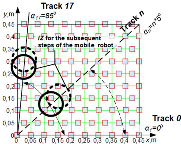
Figure 13: The interrogation zone and the limit of robot movement
