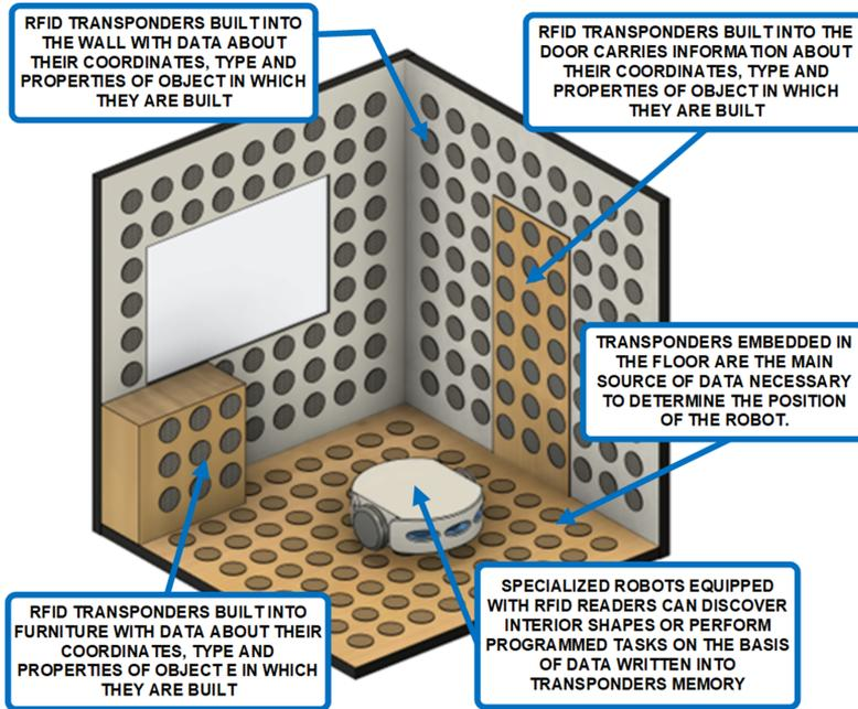
Figure 1: An example of the use of RFID grid in closed spaces
