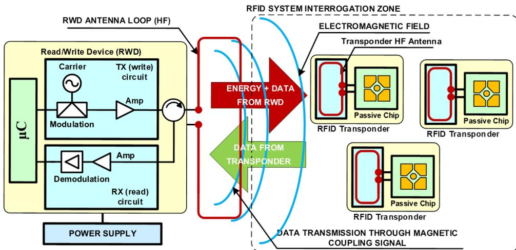
Figure 2: General diagram of the inductive coupled RFID identification system
