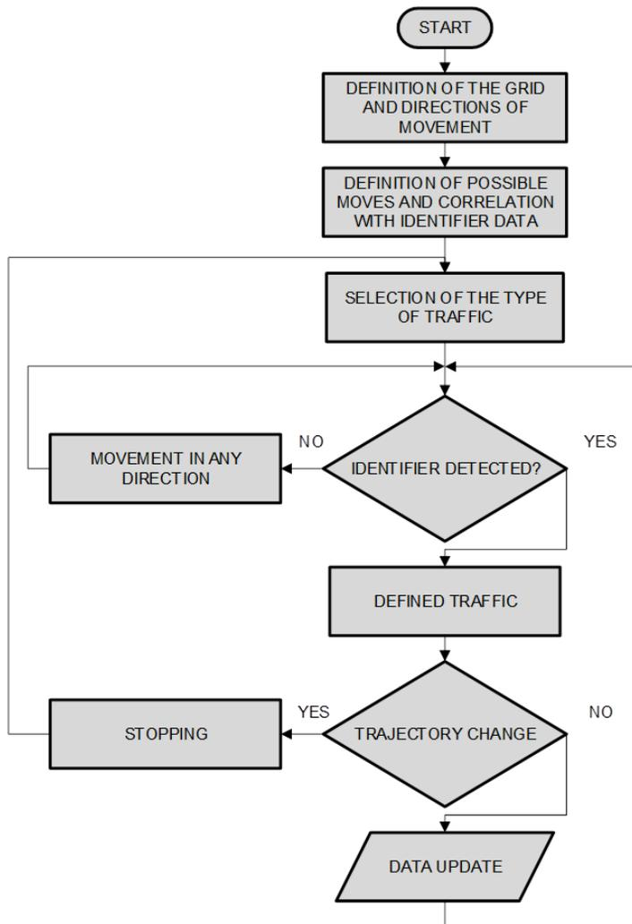
Figure 11: Algorithm for determining the movement trajectory
