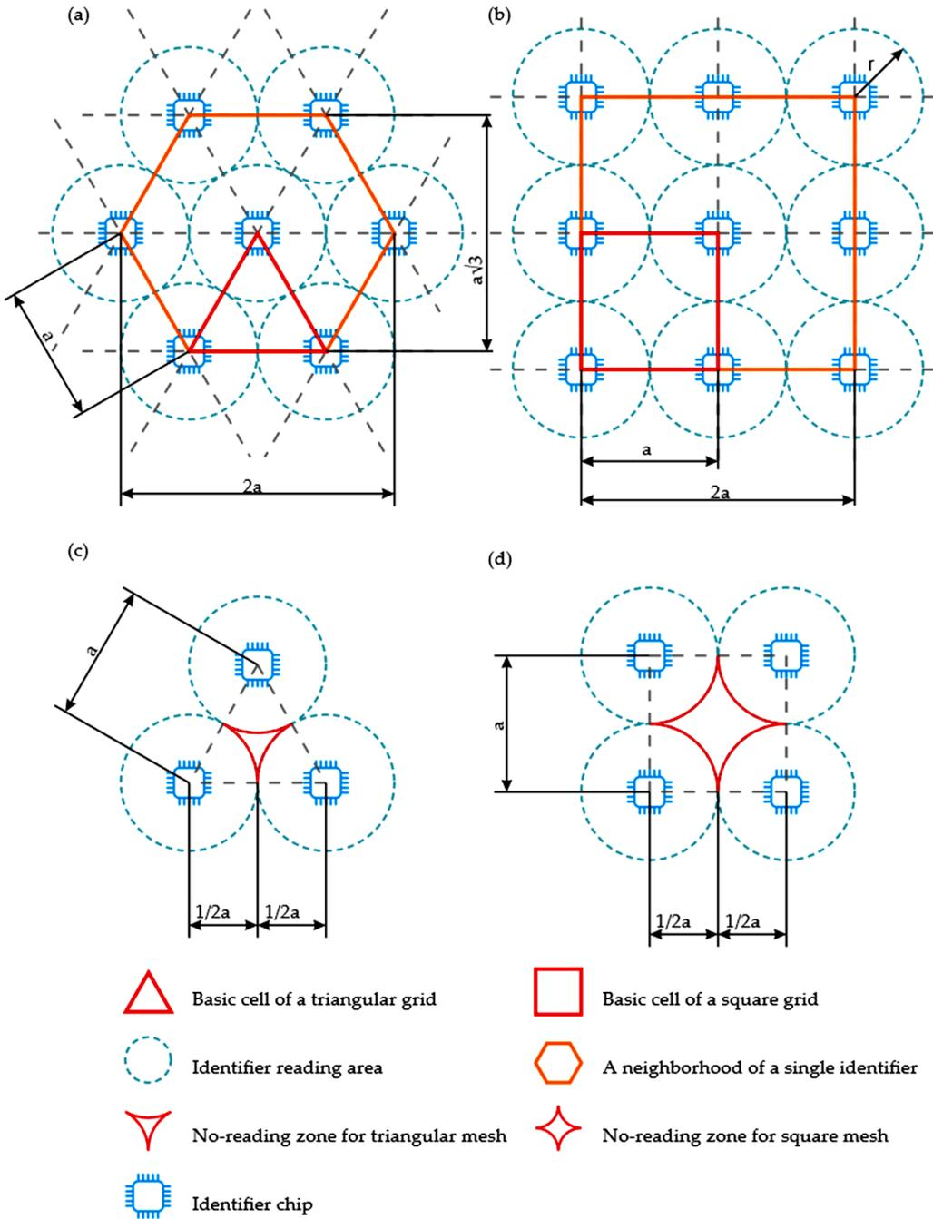
Figure 5: Basic RFID transponders: (a) triangular grid, (b) square grid, (c) no-read zone of the triangular grid, (d) no-read zone of the square grid
