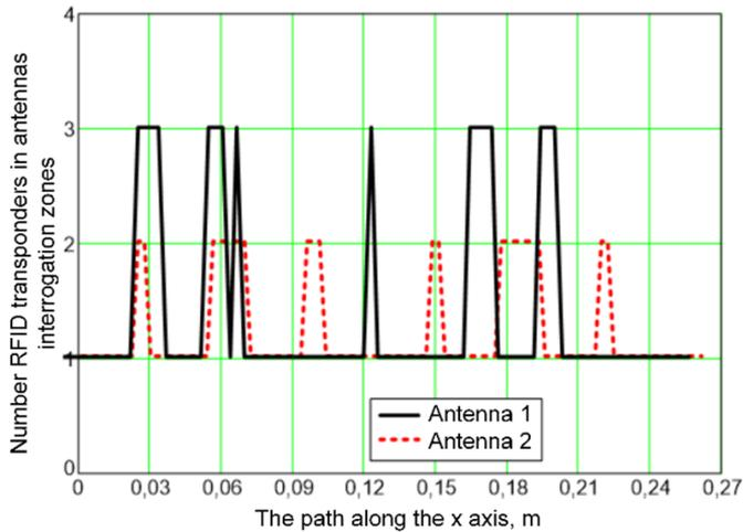
Figure 16: Number of transponders in the robot antennas interrogation zone for the triangle grid
