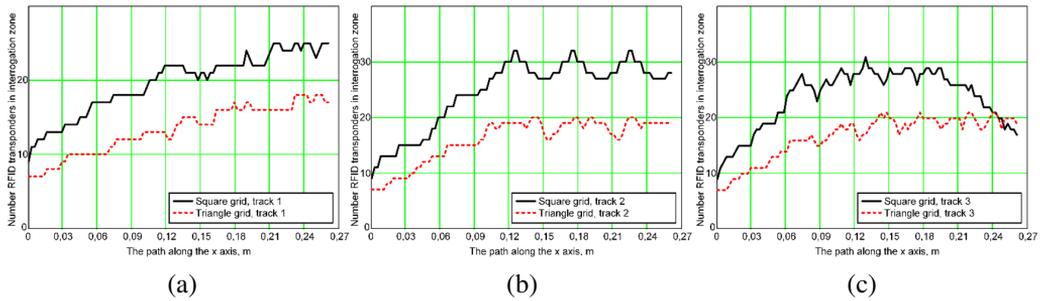
Figure 9: Number of transponders in the interrogation zone with radius  $R = 0.15$  m
