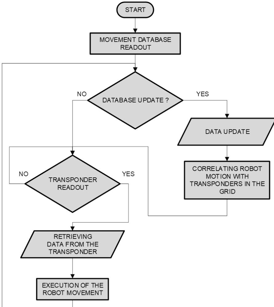
Figure 10: Robot Navigation and Mapping Algorithm
