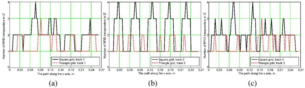
Figure 8: Number of transponders in the interrogation zone with radius  $R = 0.04$  m
