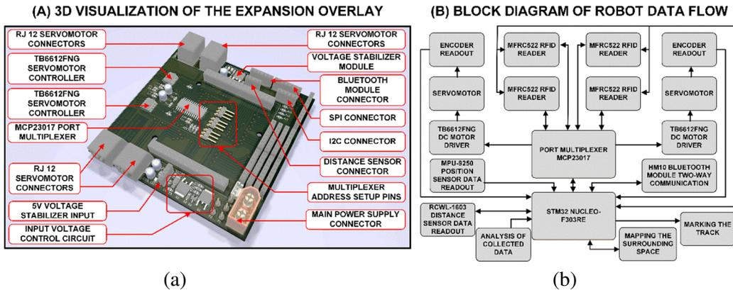
Figure 4: (a) 3D visualization of the extension board, top view, (b) a simplified block diagram of data flow in the robot control program
