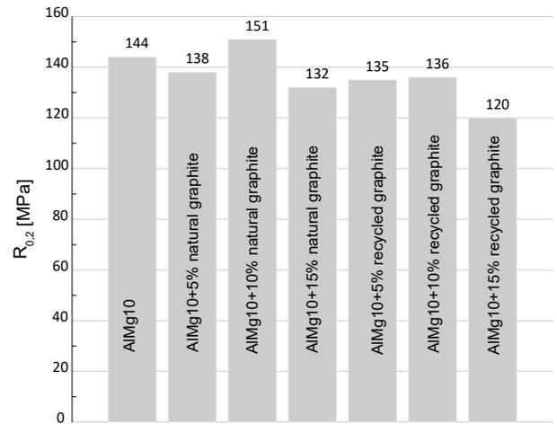
Fig. 7. Yield strength of the tested materials
