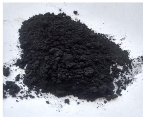
Fig. 2. Graphite from ground graphite electrodes
