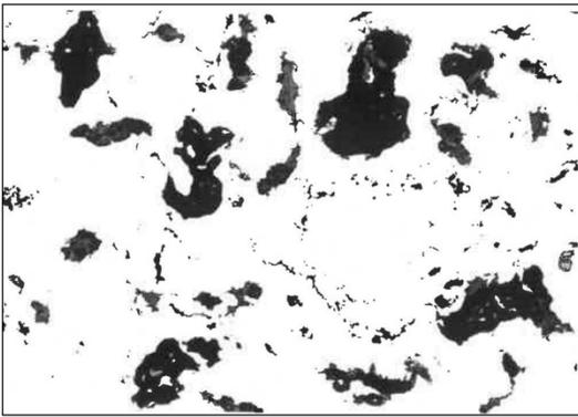
Fig. 5. Microstructure of the AlMg10 composite + 10% graphite from ground electrodes, magnification 200x
