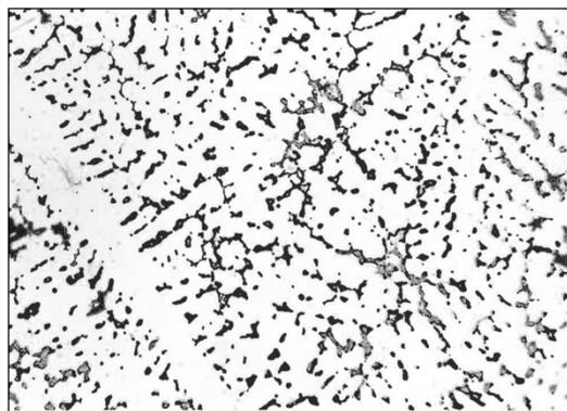
Fig. 3. Microstructure of the AlMg10 matrix alloy, magnification 200x
