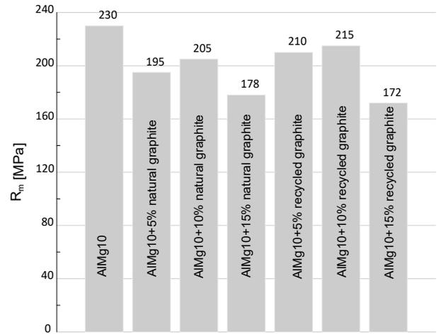
Fig. 6. Tensile strength of the tested materials
