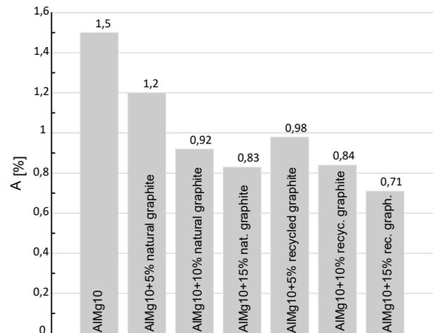
Fig. 8. Elongation of the tested materials
