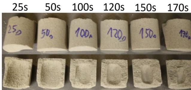
Fig. 3. Shell formation depending on curing time
