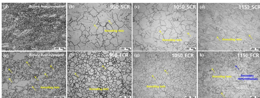
Fig. 2. Optical micrographs of hot forged Inconel 625 before and after heat treatment according to cooling rate: (a and e) before heat treatment after hot forging, after heat treatment (b)  $950^\circ\text{C}$ \_SCR, (c)  $1050^\circ\text{C}$ \_SCR, (d)  $1150^\circ\text{C}$ \_SCR, (f)  $950^\circ\text{C}$ \_FCR, (g)  $1050^\circ\text{C}$ \_FCR and (h)  $1150^\circ\text{C}$ \_FCR
