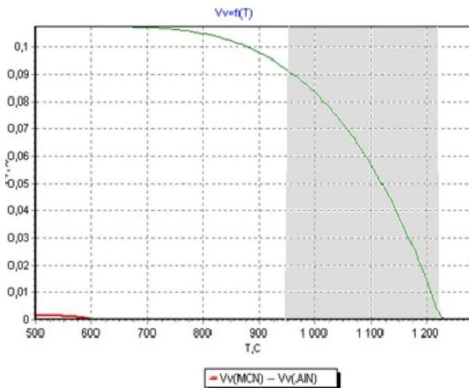
Fig. 19. Theoretical solubility curve of aluminum nitride in a ferrite matrix determined for the test steel based on the chemical composition heat No. 1
