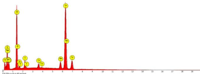
Fig. 7. Results from EDS: nitride inclusion: EDS spectrum
