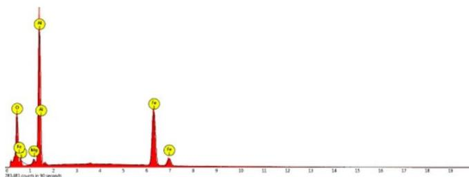
Fig. 3. Results from EDS: oxide inclusions EDS spectrum
