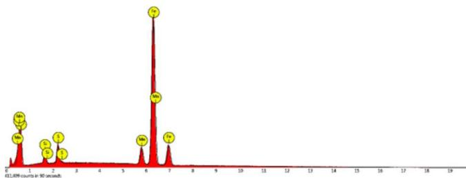
Fig. 5. Results from EDS: sulfide inclusion: EDS spectrum
