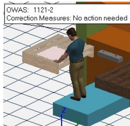
Fig. 11. Placing a metal sheet on a pallet after ergonomic intervention
