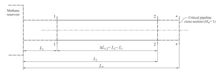
Figure 1: Fanno pipeline diagram with marked sections  $L_1$ ,  $L_2$ , and  $L_*$ .
