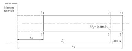
Figure 5: Diagram of section 3-3 location in Fanno flow.
