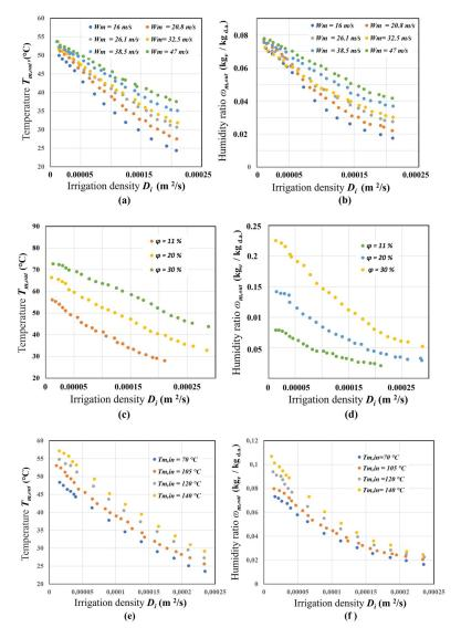
Figure 3: Outlet temperature and humidity ratio of the air-water vapour mixture versus irrigation density for different values: (a), (b) velocity of the AWVM; (c), (d) vapour content of the AWVM; (e), (f) initial temperature of the AWVM.
