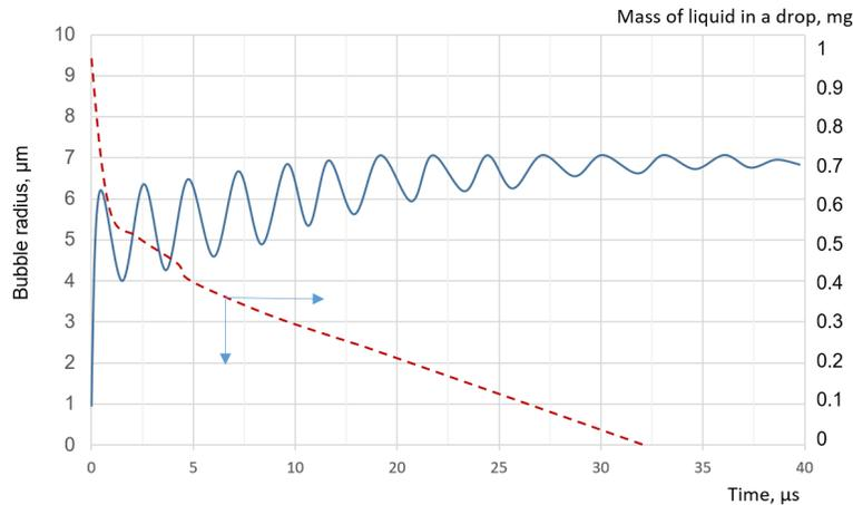
Figure 5: Change in the mass of the droplet  $m = f(\tau)$  due to evaporation into the bubble and variation in the size of the vapour bubble  $R = f(\tau)$  during the explosive boiling of the droplet: solid line –  $m = f(\tau)$ ; dashed line –  $R = f(\tau)$ .
