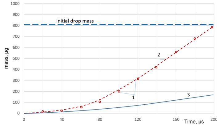
Figure 3: Change in the mass of vapour in a bubble as a result of the evaporation of liquid from a drop into the bubble during the explosive boiling of the drop.
