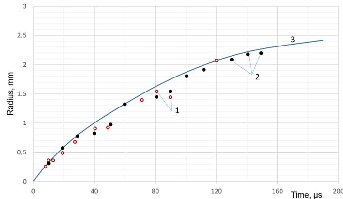
Figure 1: Changes in the radius of a vapour bubble during the explosive boiling of a liquid drop (comparison of experimental results 1 and 2, according to [51] and [52], respectively, with calculations using our model – curve 3).
