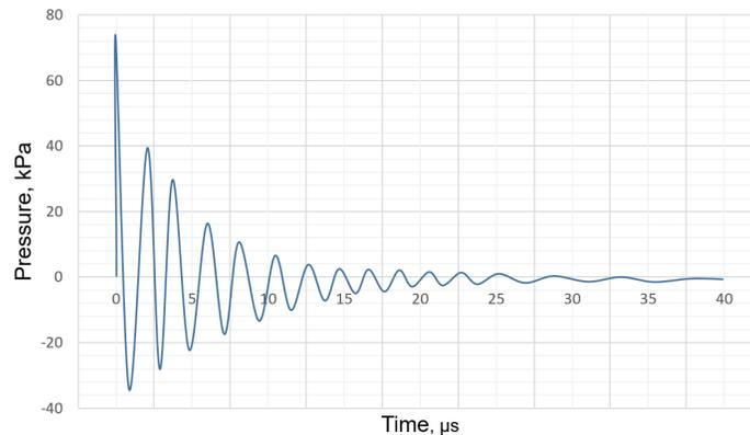
Figure 4: Change in the pressure in the liquid at a distance of 6 mm from the centre of the vapor bubble during the explosive boiling of a drop until its destruction [52].
