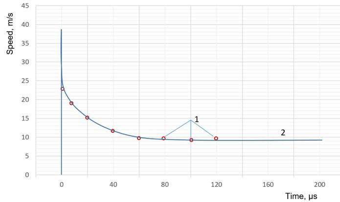
Figure 2: The speed of radial motion of the wall of a bubble growing during explosive boiling of a liquid drop: comparison of experimental results (points 1) [52] with calculated data using the model (curve 2).
