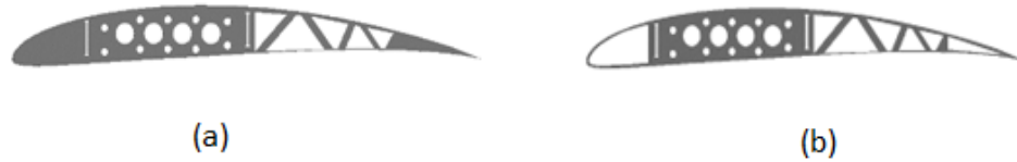
Fig. 7. Comparison of the wing rib design: (a) original (b) topology optimized
