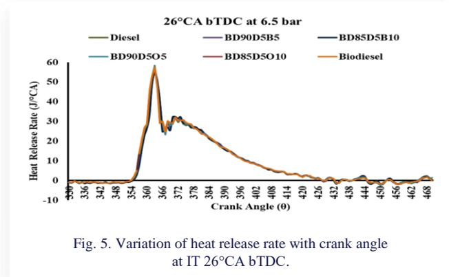
Fig. 5. Variation of heat release rate with crank angle at IT 26°CA bTDC.
