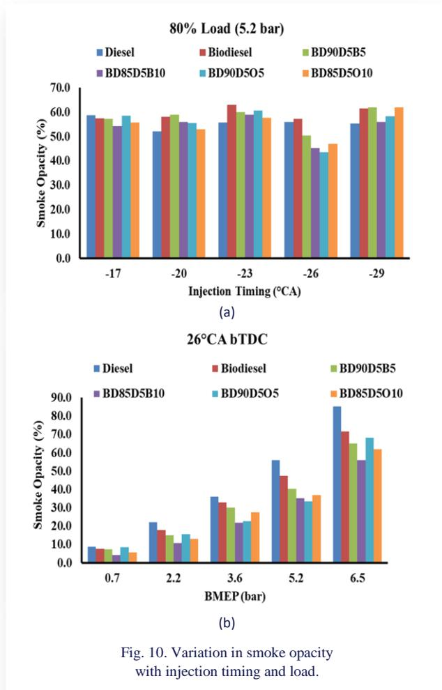
Fig. 10. Variation in smoke opacity with injection timing and load.
