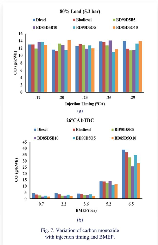
Fig. 7. Variation of carbon monoxide with injection timing and BMEP.
