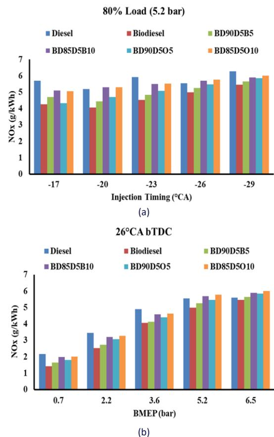
Fig. 9. Variation of oxides of nitrogen with injection timing and BMEP.
