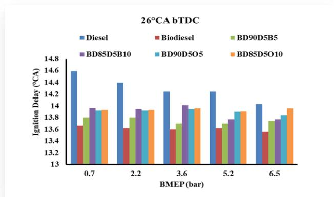
Fig. 6. Variation in ignition delay with BMEP.
