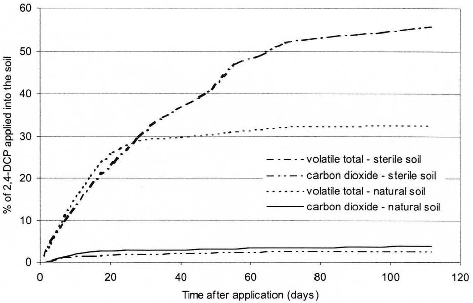
Fig. 3. Volatile compounds evolved from the soil treated with 2,4-dichlorophenol
