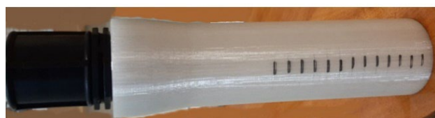
Fig. 3. Geometry of the shroud pipe (ladle shroud) used in the water model tests
