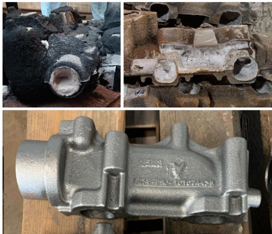
Fig. 9. Clockwise from top left: Castings after shakeout, after degating and after shot blasting
