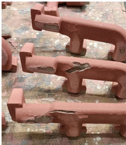
Fig. 8. Cracked cores after drying
