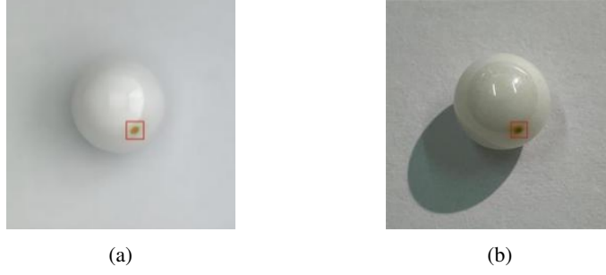
Fig. 2. Collected defective ceramic ball sample images. (a) using coaxial light source; (b) without using coaxial light source.
