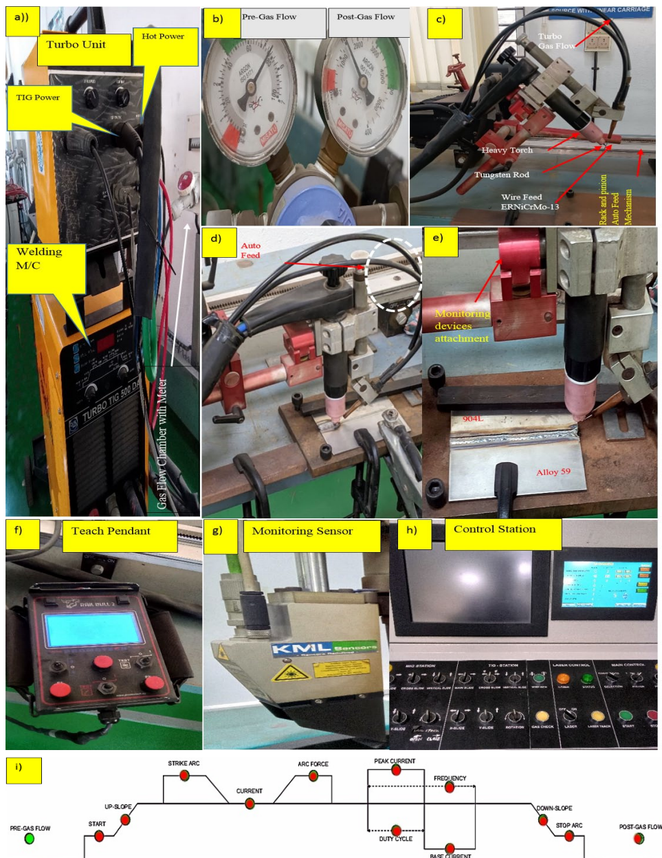
Fig. 2. Hot wire TIG welding machine working (a to h) Machine set-up; i) Process sequence
