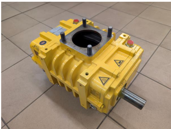
Fig. 7. View of the selected rotary blower.
