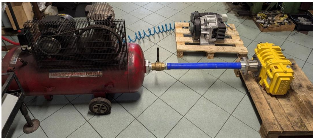
Fig. 10. Preliminary tests of the selected devices during their operation in a reverse cycle.
