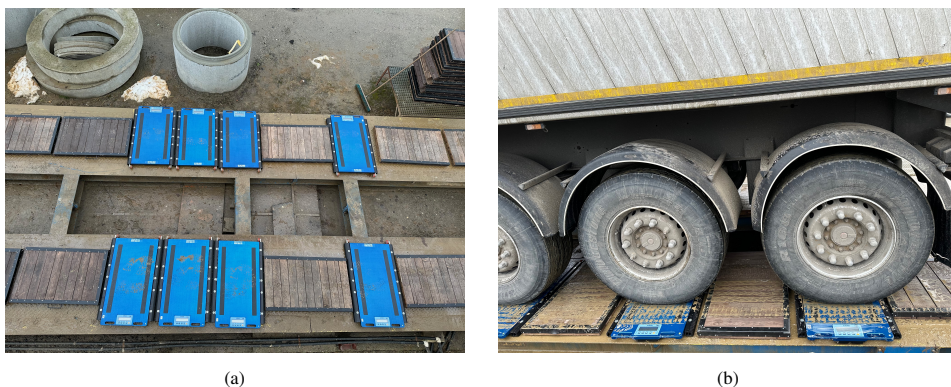
Fig. 1. Arrangement of the station for simultaneous weighing of vehicles on the platform scale and portable scales.
