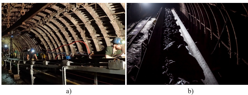
Fig. 2. Belt conveyors transport: a) for people, b) for output [6,7]
