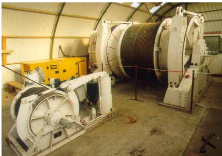
Fig. 4. Transport using rope winch (hauling)
