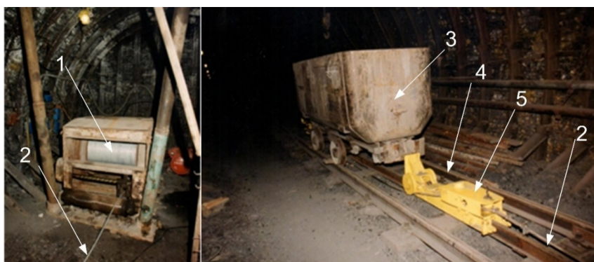
Fig. 5. Transport system with a rope winch in an inclined underground excavation
