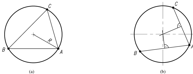
Fig. 1. Illustration of different models for coordinate measurement of a circle radius: a) radius calculated as the radius of a circle circumscribed on a triangle, b) centre of the circle determined as the intersection point of the perpendicular bisectors of the triangle's sides.
