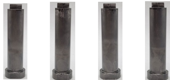
a) Sample C-1 b) Sample C-2 c) Sample 3D-1 d) Sample 3D-2 Fig. 2. Components for test sample production – conventional (a, b) and additive (c, d) manufacturing
