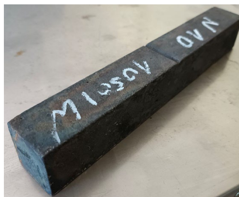
Fig. 4. Scheme (a) and example view (b) of the impact test specimen according to PN-EN 15689
