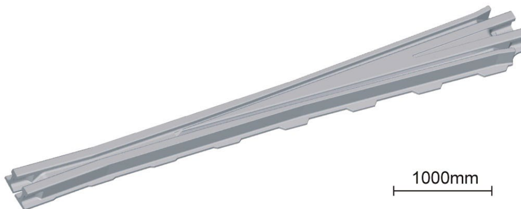
Fig. 2. Scheme of monoblock frog R500 (R – turnout radius in meters)
