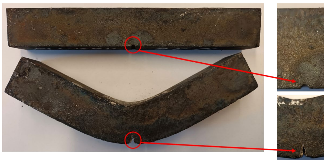
Fig. 6. Specimen before (top) and after (bottom) impact bending test, showing the crack at the U-notch subjected to measurement
