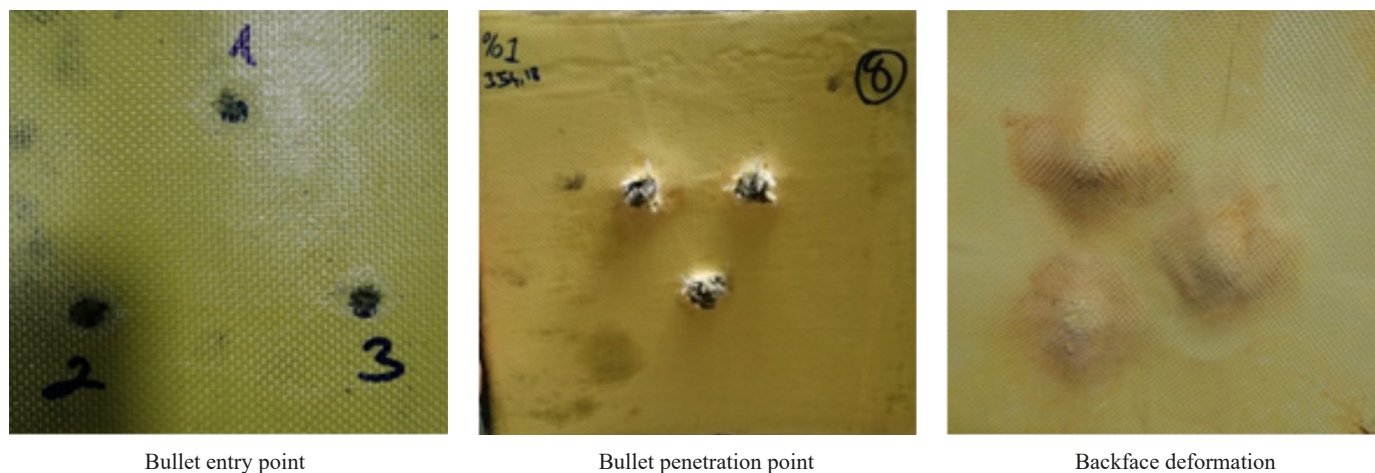
Fig. 12. Movement of bullet on ballistic plates
