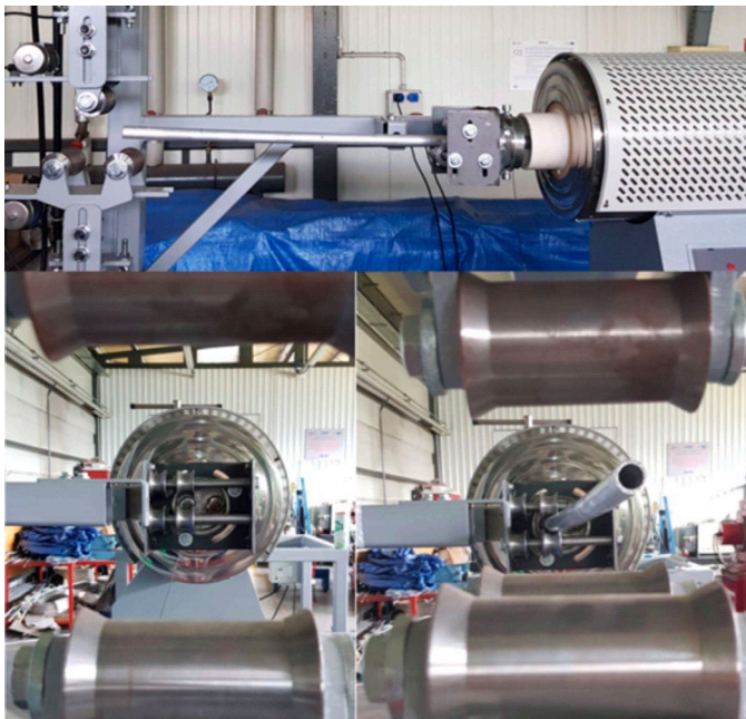
Fig. 12. Examination of a \text{Ø}25 \times 3 mm tube without a gripping system. Shots before and during the examination
