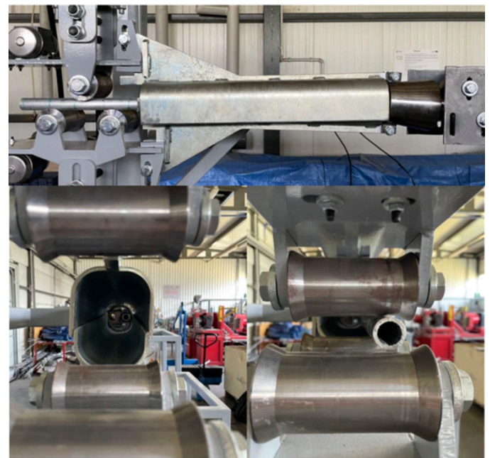
Fig. 13. Examination of a \text{Ø}25 \times 3 mm tube with a gripping system. Shots before and during the examination
