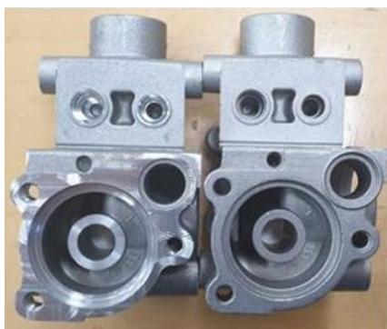
Fig. 4. Comparison of parts before (right) and after (left) machining
