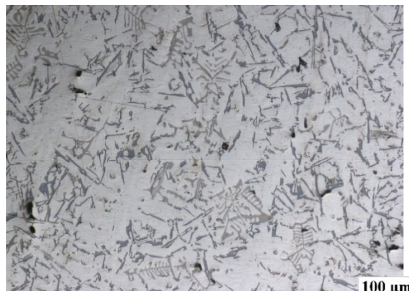
Fig. 8. Microstructure of undegassed EN AC-46000 alloy from the TDA probe
