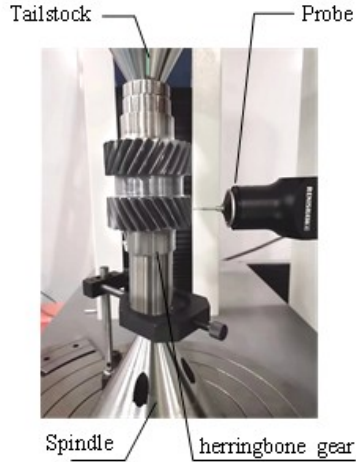
Fig. 7. GMC650 and the pinion gear under test.
