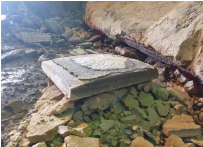
Fig. 7. Retrieved impact pad after casting, showing preserved shape and minimal surface degradation
