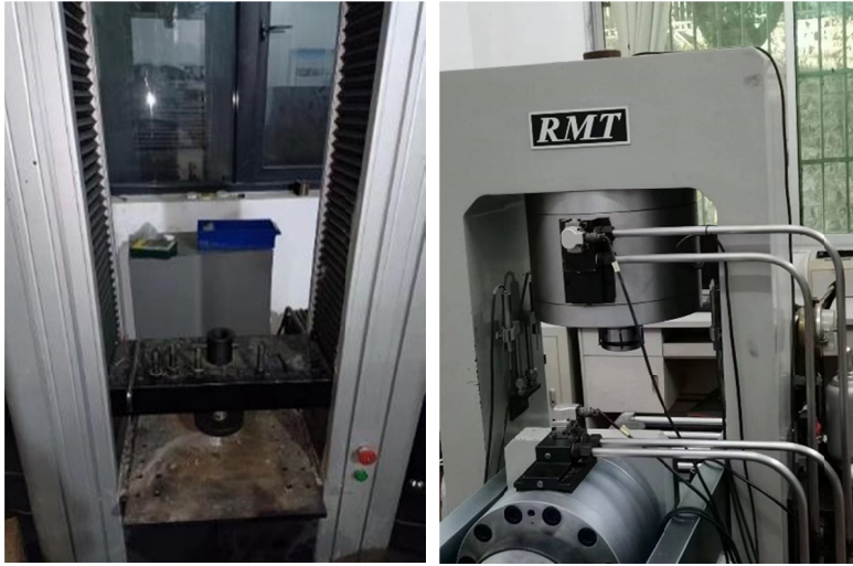
Fig. 4. Conventional rock mechanical test machines: (a) Compression test machine, (b) Triaxial compression test machine
