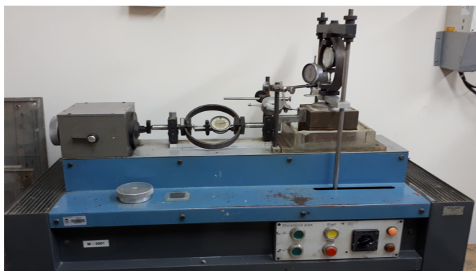
Fig. 2. General view of the AB2A direct shear apparatus and shear box (photo credit: R. Wojtaszek)
