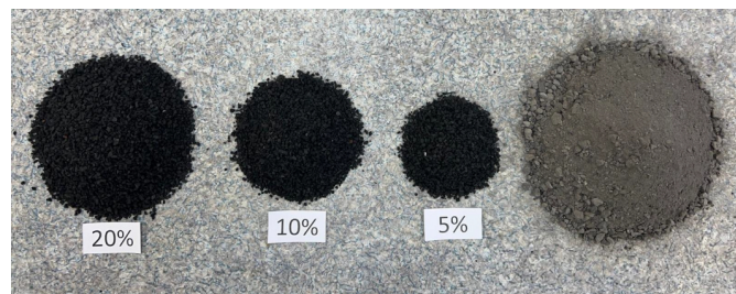
Fig. 1. Comparison of the colliery spoils sample with the applied crumb rubber additive
