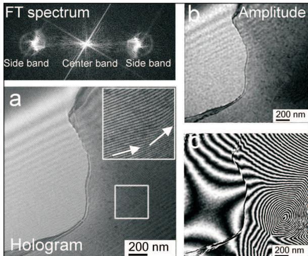
Fig. 26. Electron holography of the as-grown FeCo-based alloy: a) Electron hologram; b) Reconstructed amplitude and c) phase images of FeCo-based alloys. The phase image has been amplified by two times
