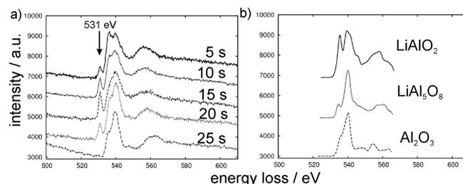
Fig. 19. Time-resolved ELNES of  $\gamma$ - $\text{LiAlO}_2$ : a) Experimental O-K edge spectra acquired at a focused electron beam of 1 nm in diameter at 200 kV accelerating voltage at different irradiation time; b) simulated ELNES of O-K edge for different phases
