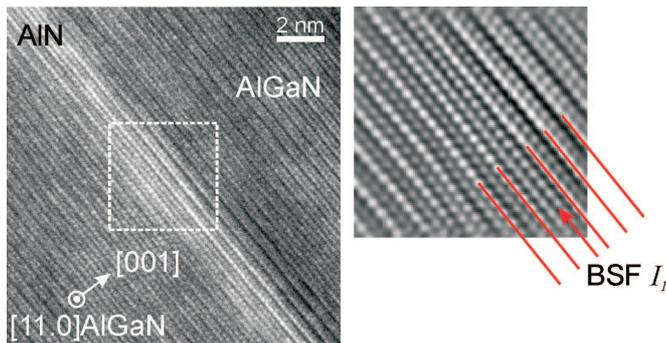
Fig. 10. HRTEM image of a thin AlN layer in an AlN/(Al,Ga)N superlattice with a Fourier filtered fragment showing periodic image of the wurtzite crystal structure (... ABAB...) containing an  $I_1$  type basal plane stacking fault (... ABABCBC...)
