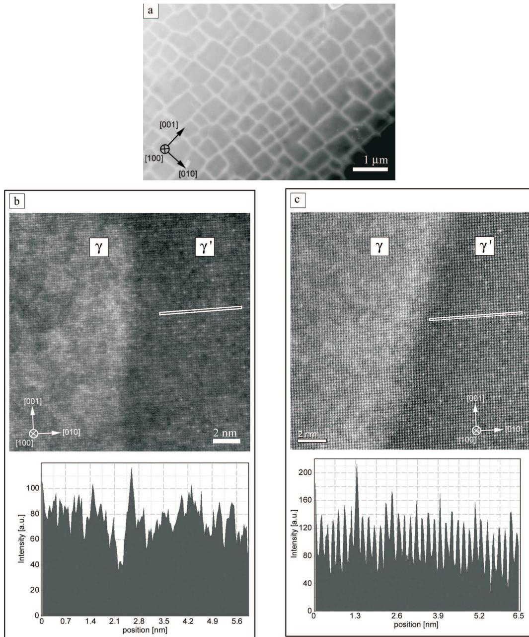
Fig. 5. HAADF imaging of nickel-base superalloy (CMSX-10): a) HAADF overview image, b) conventional high-resolution HAADF image (TEM/STEM JEOL JEM 2200FS (FEG, 200 kV, probe size: 0.14 nm)) of the  $\gamma/\gamma'$  interface and intensity profile along the marked line, c)  $C_s$ -corrected high-resolution HAADF image (TEM/STEM JEOL 2100F/ $C_s$ -corrector (FEG, 200 kV, probe size: 0.1 nm)) of  $\gamma/\gamma'$  interface and intensity profile along the marked line
