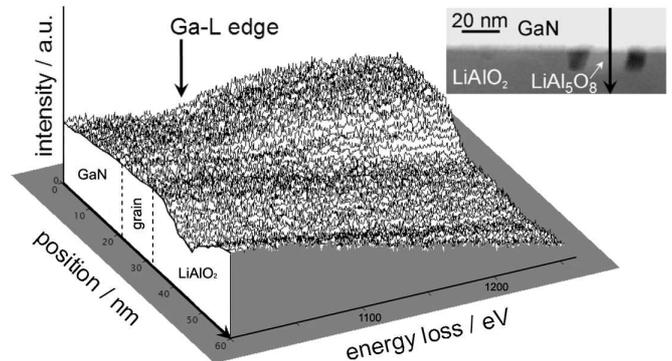
Fig. 17. STEM EELS line scan across the  $\text{GaN}/\text{LiAlO}_2$  interface and the corresponding HAADF STEM image. The scan direction is shown by an arrow. Energy loss spectra show Ga-L edge at 1115 eV revealing the Ga distribution
