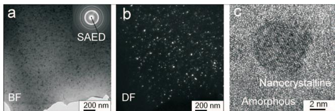
Fig. 21. Microstructure of  $(\text{Fe}_{0.5}\text{Co}_{0.5})_{80}\text{Nb}_4\text{B}_{13}\text{Ge}_2\text{Cu}_1$  nanocrystalline soft-magnetic alloy: (a) bright-field TEM image (inserted: diffraction pattern); (b) dark-field TEM image; (c) HRTEM image
