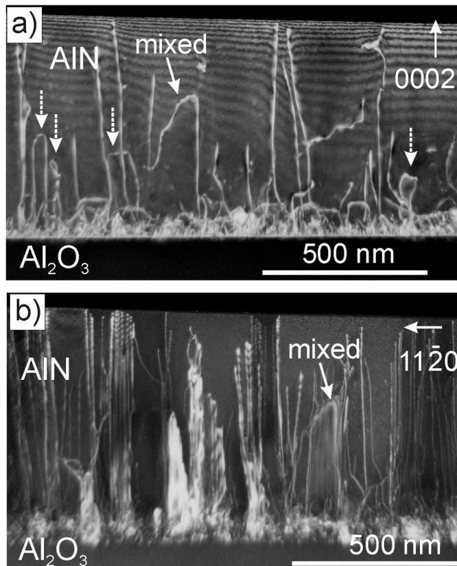
Fig. 8. Cross-sectional dark-field images of approximately the same specimen area obtained under two-beam diffraction conditions using a)  $g = 0002$  and b)  $g = 11-20$ . The images show a) screw and b) edge dislocations. Dislocations with a mixed character are visible in both images. Dashed arrows in a) show annihilation of some dislocations with a screw component of the Burgers vector
