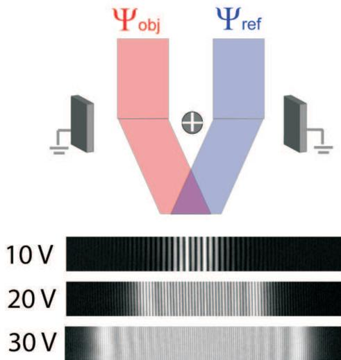
Fig. 25. Basic principle of off-axis electron holography
