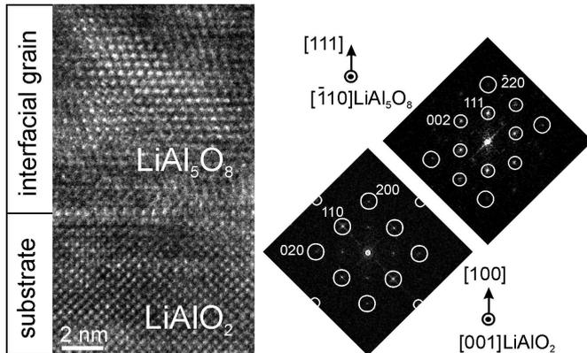
Fig. 15. HRTEM image (left) of an interfacial crystallite and its interface to the  $\text{LiAlO}_2$  substrate. Two Fourier spectra (right) which were calculated from the substrate and the crystallite HRTEM images. Diffraction simulations (circles) correspond to the  $[001]$   $\text{LiAlO}_2$  zone axis (which was used for calibration of distances) and to  $[\bar{1}10]$   $\text{LiAl}_5\text{O}_8$  zone axis
