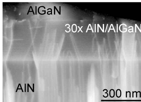
Fig. 9. Cross-sectional ADF STEM image of AlN/(Al,Ga)N superlattice grown on AlN buffer layer. Threading dislocations of all types (screw, edge, mixed) are visible as bright lines
