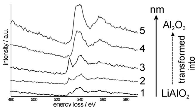
Fig. 20. ELNES of the O-K edge extracted from the EELS line scan (shown in Fig. 16) carried out through a  $\text{LiAlO}_2$  region. The spectra numbering corresponds to the notations marked in Fig. 16
