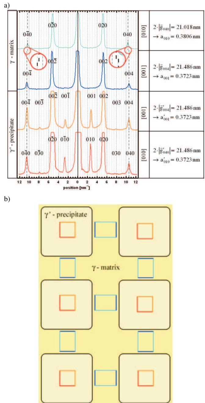
Fig. 3. Interpretation of the diffraction patterns (Fig. 2b): a) intensity profiles of the reflections along the [010] and [001] directions. The measured  $\vec{g}$  vectors and calculated lattice parameter  $a$  are listed in the table, b) schematic presentation of arrangement and strain state of the unit cells
