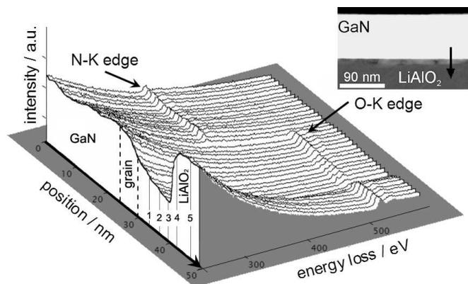
Fig. 16. STEM EELS line scan across the  $\text{GaN}/\text{LiAlO}_2$  interface containing interfacial grains. The scan direction is shown in the inserted STEM image by an arrow. Energy loss region between 220 and 600 eV contains N-K edge at 401 eV and O-K edge at 532 eV. The numbers 1 to 5 mark positions of the spectra used for ELNES investigations discussed in Fig. 20
