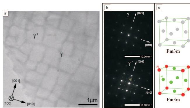
Fig. 2. Structure analysis of nickel-base superalloy (CMSX-10): a) TEM absorption contrast image, b) SAED patterns of the  $\gamma$ - and  $\gamma'$ -phases, c) corresponding structure models
