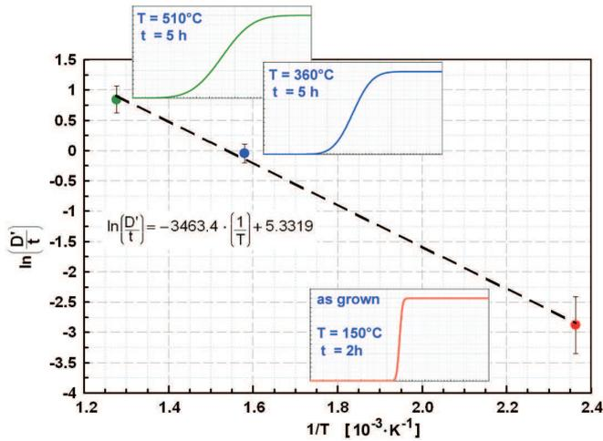
Fig. 7. Arrhenius plot of the diffusion coefficient  $D$  as a function of temperature. The dots are calculated from the corresponding Cd concentration profiles and annealing parameters (see images in rectangles). The dashed line is gained by linear regression
