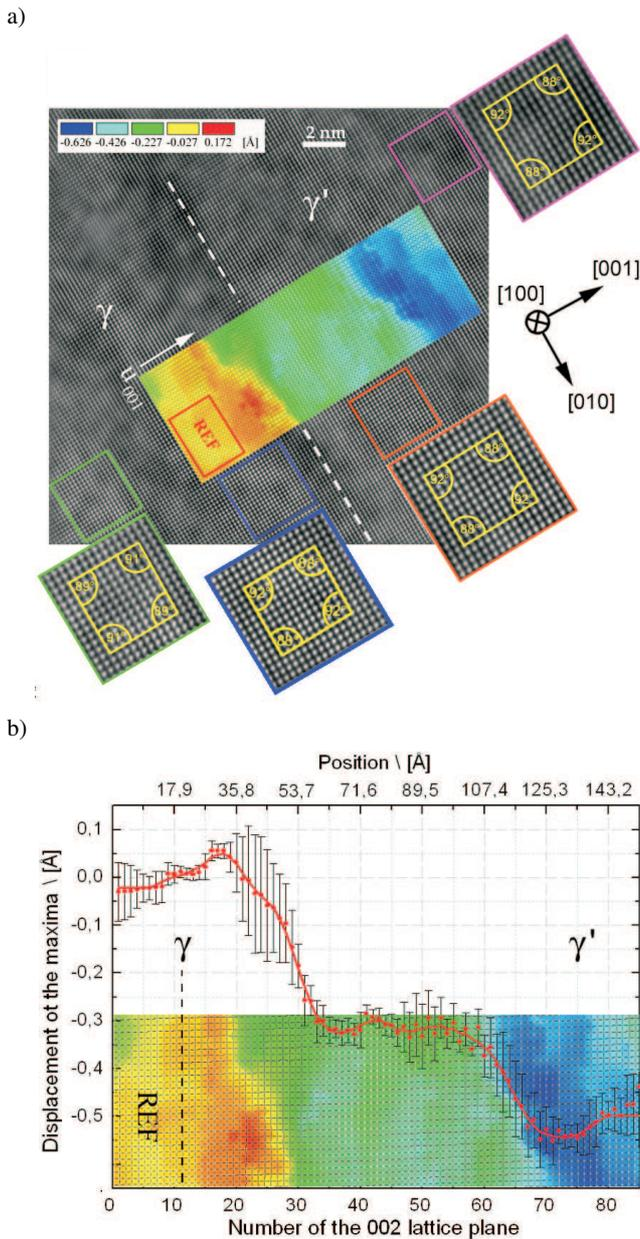
Fig. 4. Quantitative HRTEM of nickel-base superalloy (CMSX-10): a) Fourier-filtered HRTEM image of  $\gamma/\gamma'$  interface analysed by DALI. The colour-coded map represents the displacement of the atom columns in [001] direction compared to the reference lattice (REF), b) one-dimensional plot of displacements  $u_{001}$  of the (002) lattice planes with respect to the REF given in a). The values are averaged along the (002) lattice planes
