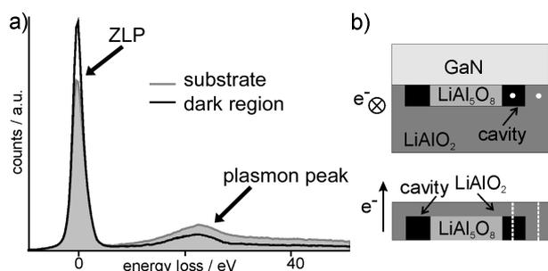
Fig. 18. Geometry of  $\text{LiAl}_5\text{O}_8$  grains: a) Low-loss spectrum region containing information on elastically scattered electrons and the plasmon losses. A higher ZLP-to-plasmon intensity ratio in the dark region corresponds to a smaller specimen thickness. b) Sketches of the sample structure visualizing the electron beam position used for the measurements shown in (a): cross-sectional view (top) and top-view without the GaN layer (bottom)
