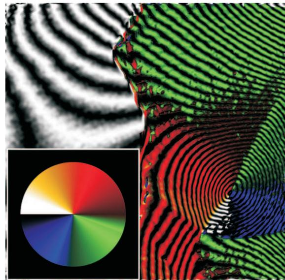
Fig. 27. Colour-coded magnetic flux distribution in FeCo-based soft-magnetic alloys. The directions of magnetic flux are indicated by the colour-wheel inserted at bottom left. Image size:  $1.82 \mu\text{m} \times 1.82 \mu\text{m}$
