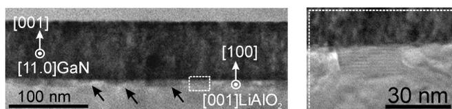
Fig. 14. Cross-sectional TEM micrograph of a GaN layer on LiAlO<sub>2</sub> substrate. A number of crystallites appearing at the GaN/LiAlO<sub>2</sub> interface are marked by arrows. An interfacial region marked by the dashed line is shown on the right at a higher magnification
