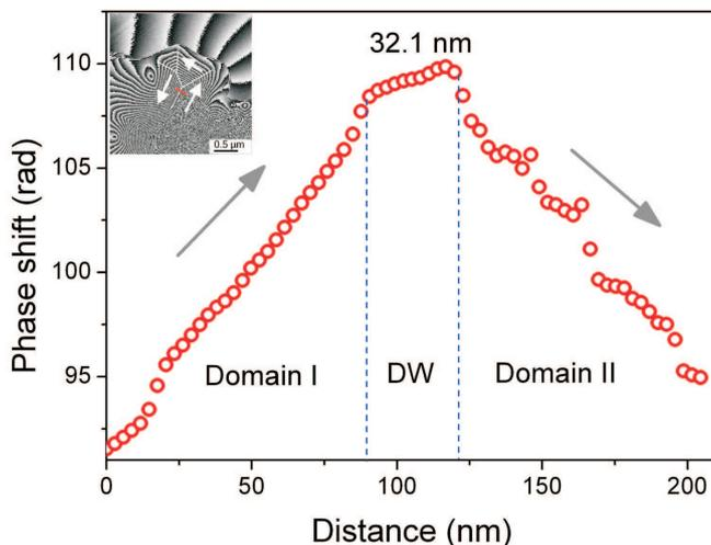
Fig. 28. Unwrapped phase line profile perpendicular to a 180° domain wall. The relatively flat part in the center region clearly reveals the width of domain wall
