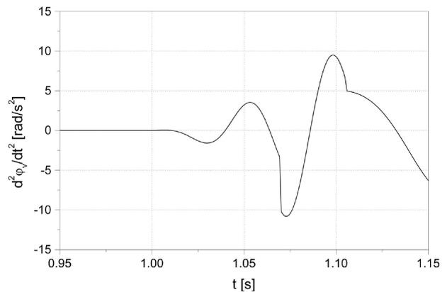
Fig. 9. Angular acceleration of the turret in the tilt motion during the missile launch
