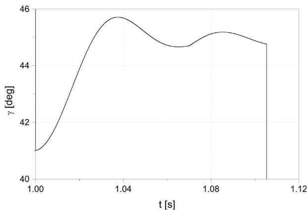
Fig. 12. Direction angle of the missile linear velocity vector  $\gamma$  during a launch
