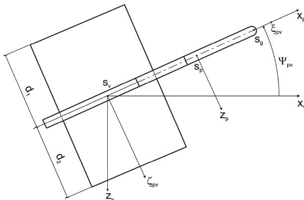
Fig. 3. Top view of the turret-and-missile model
