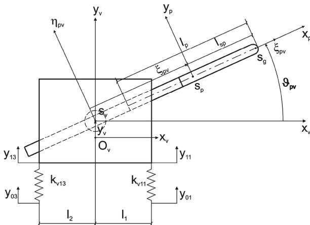
Fig. 2. Side view of the turret-and-missile model
