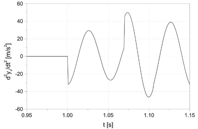
Fig. 5. Linear acceleration of the turret during the missile launch
