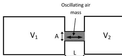
Fig. 5. The two-chamber Helmholtz resonator
