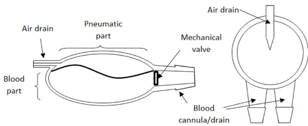
Fig. 3. Polish heart supporting device – POLVAD diagram
