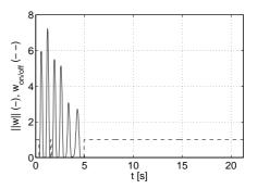
Fig. 10. Experiment 1: module of the collision avoidance component of the control (||w||) and logical value that indicates collision avoidance is on (value 0) off (value 1)
