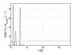
Fig. 20. Experiment 3: module of the collision avoidance component of the control (||w||) and logical value that indicates collision avoidance is on (value 0) off (value 1)
