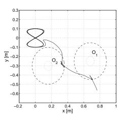
Fig. 21. Experiment 4: trajectory of the robot and desired trajectory on the (x, y) plane
