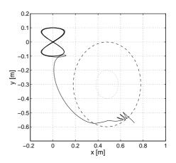
Fig. 11. Experiment 2: trajectory of the robot and desired trajectory on the (x, y) plane
