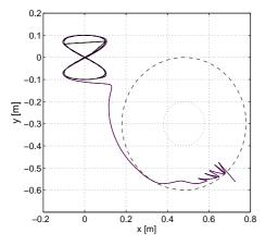
Fig. 6. Experiment 1: trajectory of the robot and desired trajectory on the (x, y) plane
