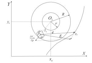
Fig. 3. Robot is in the repel area of obstacle  $O_1$ . Modified position error E is computed as a difference between the tracking error and the gradient of the APF
