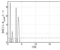
Fig. 25. Experiment 4: module of the collision avoidance component of the control (||w||) and logical value that indicates collision avoidance is on (value 0) off (value 1)
