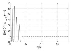
Fig. 15. Experiment 2: module of the collision avoidance component of the control (||w||) and logical value that indicates collision avoidance is on (value 0) off (value 1)
