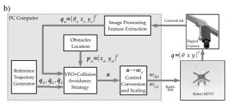
Fig. 5. Mobile robot MTV3 used in experiments (a) and a block schema of the control system (b)
