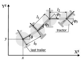
Fig. 1. Illustration of three on-axle trailers driven by one unicycle-like tractor
