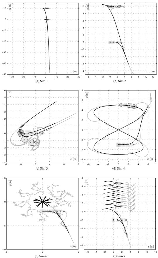
Fig. 10. Path describing position of the last trailer ( $\blacksquare$ ) and the tractor ( $\blacksquare$ )
