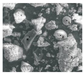
Fig. 2. E-SEM image of fly ash from co-combustion of hard coal and wood biomass, magnification ×5000.
