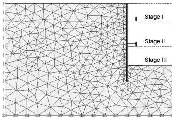
Fig. 4. Soil discretization by finite element mesh in PLAXIS program.
