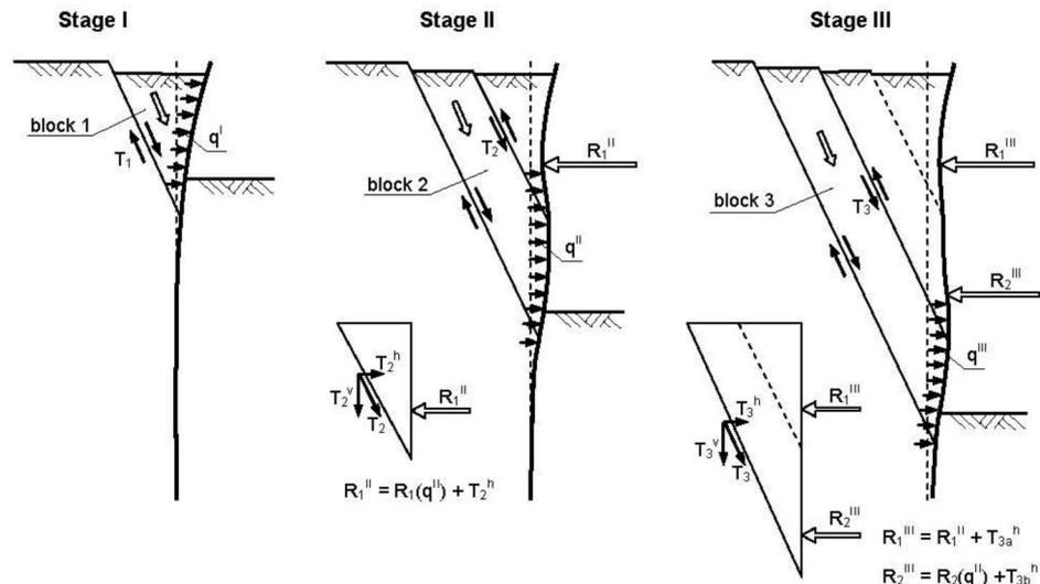
Fig. 14. A scheme of soil deformations in the area behind the wall during subsequent excavation stages.
