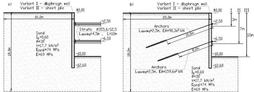
Fig. 5. Geometrical parameters of the deep excavation walls.
