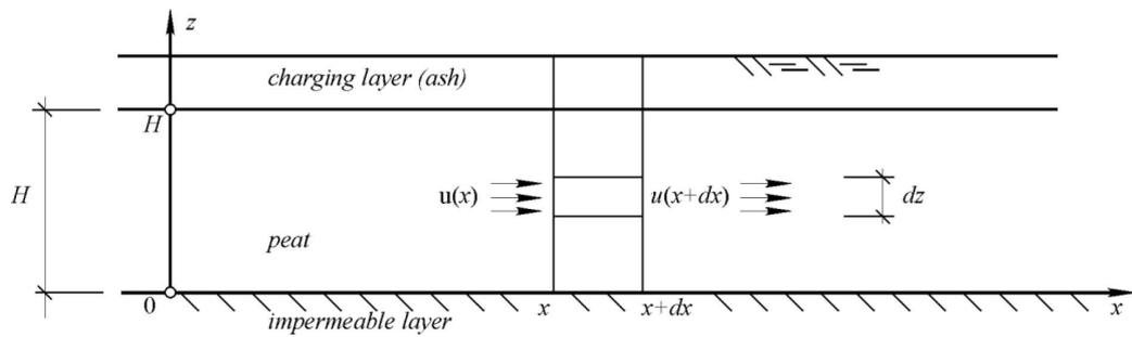
Fig. 6. Consolidation with horizontal water flow.
