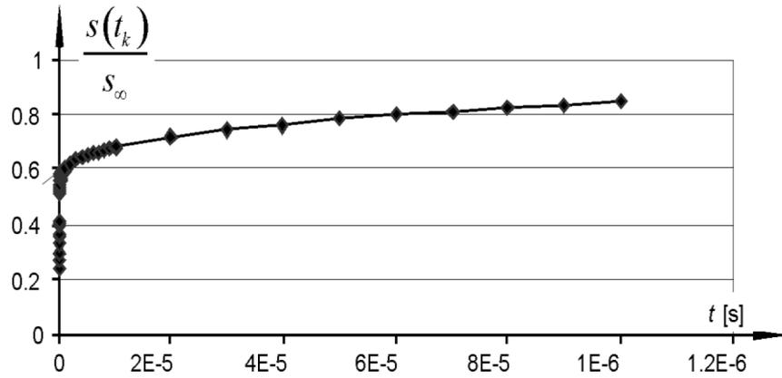
Fig. 13. Stabilization of terminal settlement [4].
