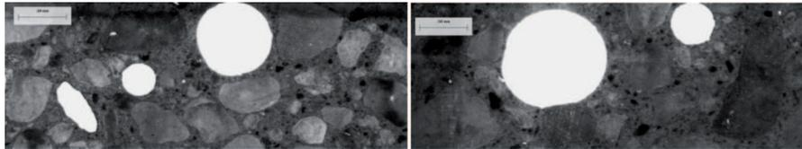
Fig. 3. The porosity characteristics of non air-entrained SCC (CEM II 32.5 R B-S;  $w/b=0,41$ ) [14].
