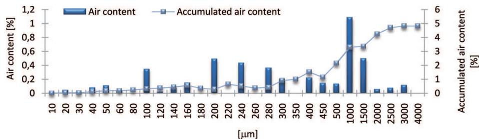
Fig. 2. The porosity characteristics of non air-entrained SCC (CEM II 32.5 R B-S;  $w/b=0.29$ ) [14].
